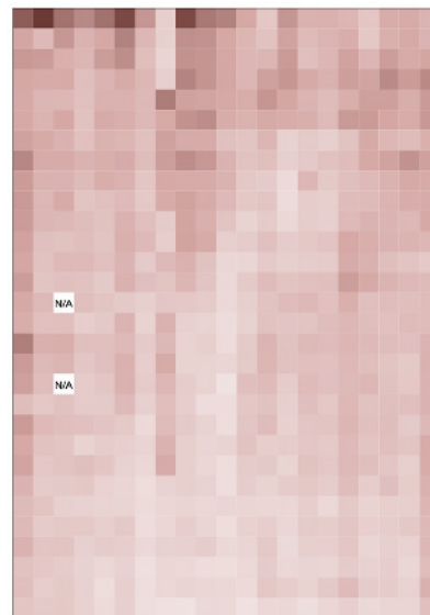
FIGURE 8 MDMB-CHMICA concentration mapping across impregnated paper showing a significant variation in concentration across the paper sheet
